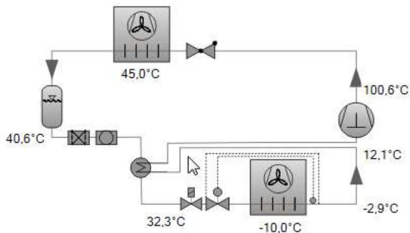
Example **dew point**: R407C // -10/45/SH after evap. 5 K total 20 K/SC inside condenser 2 K
