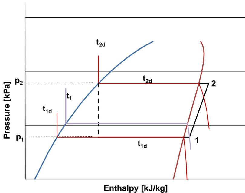
Figure 1: p–h diagram for azeotropic mixture
